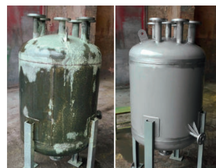
Before After Photos: Pickling of steel grade 321 (1.4541) Temp 5°C with pickling time 90 min.
