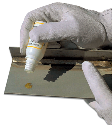
Photo : Showing easy test for differentiating stainless steel grade 304 from 316.
