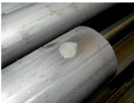
Photo: Test result showing 304 ( 1.4301 ) grade, no colour change.
