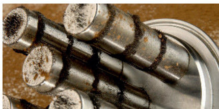
Photo: The tricky thing with free (unalloyed) iron particles is that you don't see them on the surface of stainless steel, until they start rusting in humid air and get brownish
